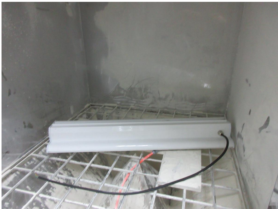
Photo 2: IP6X test of model ZL4C-150WH
