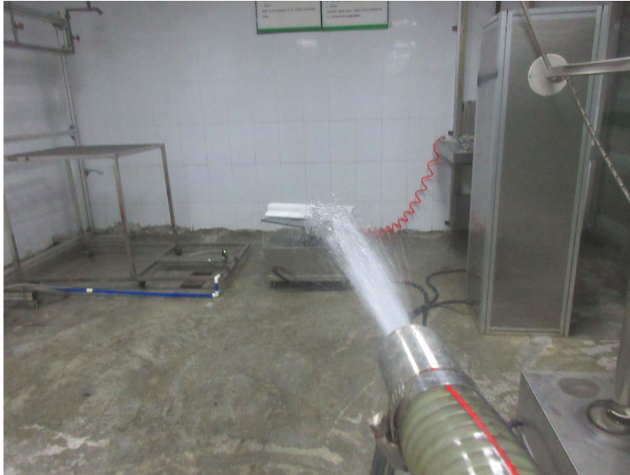
Photo 3: IPX6 test of model ZL4C-150WH
