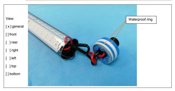
Details of: Waterproof cover at the end (the end is closed during the IP67 test)
